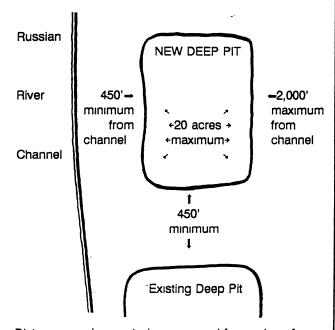
Distances and areas to be measured from edge of excavation in pre-mining surface and from ordinary high-water mark of Russian River channel.
