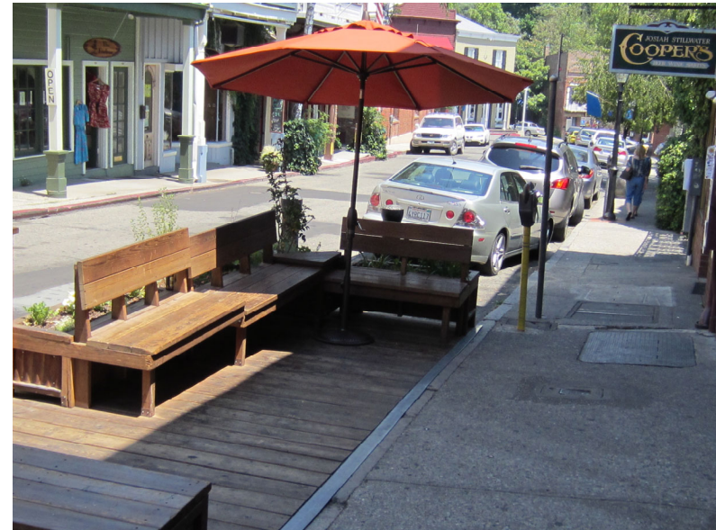
Parklets are typically small open spaces that extend sidewalks to provide public gathering spaces along streets.
