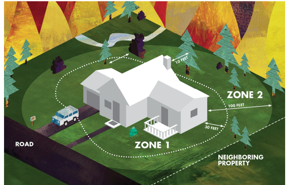
CAL FIRE identifies two defensible space zones to improve a home’s chance of surviving a wildfire. Zone 1 extends 30 feet from buildings and structures and Zone 2 extends 100 feet from buildings and structures. Section 13A-4 of the County Code identifies hazardous vegetation and combustible material abatement requirements for each zone. Image source: www.readyforwildfire.org .
