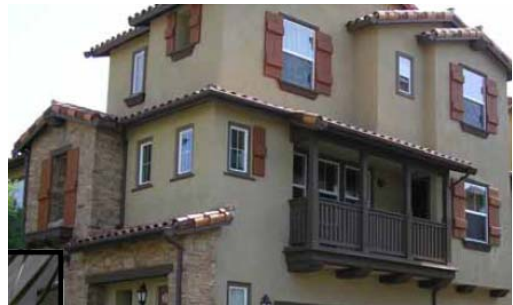
Variations in the wall plane, architectural detailing, and a combination of textures reduce the scale of the building.
