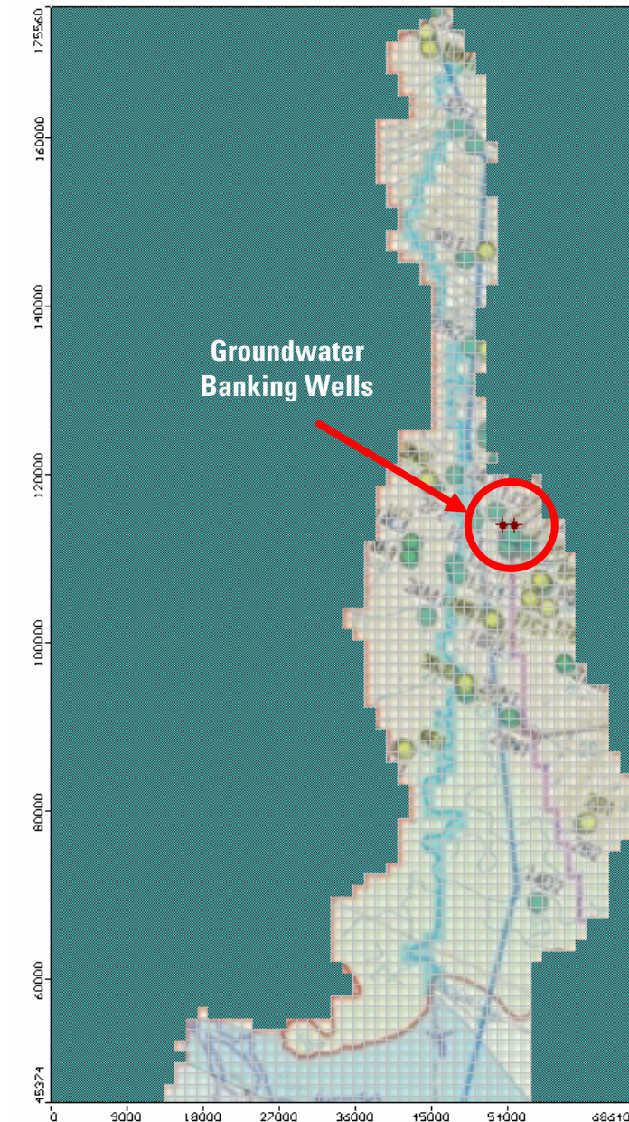
Figure 3-6 Location of Groundwater Banking Wells Represented In Model.
